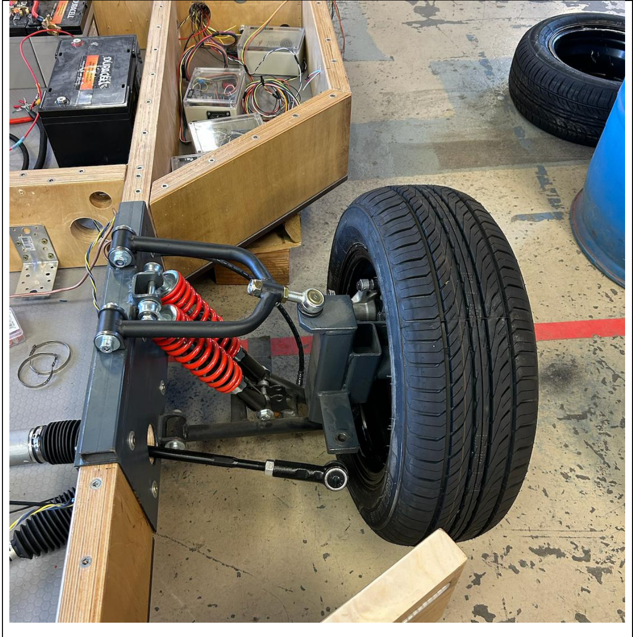
Figure 2. Current suspension and steering assembly integration state (rear corner).
